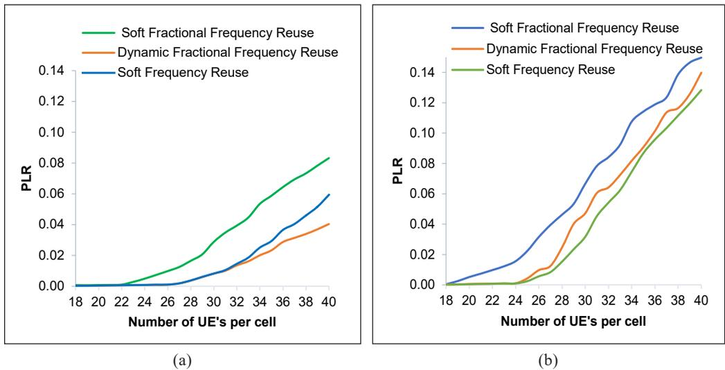
Figure 5. Packet loss ratio (PLR) for the (a) cell centre users and (b) cell edge users
