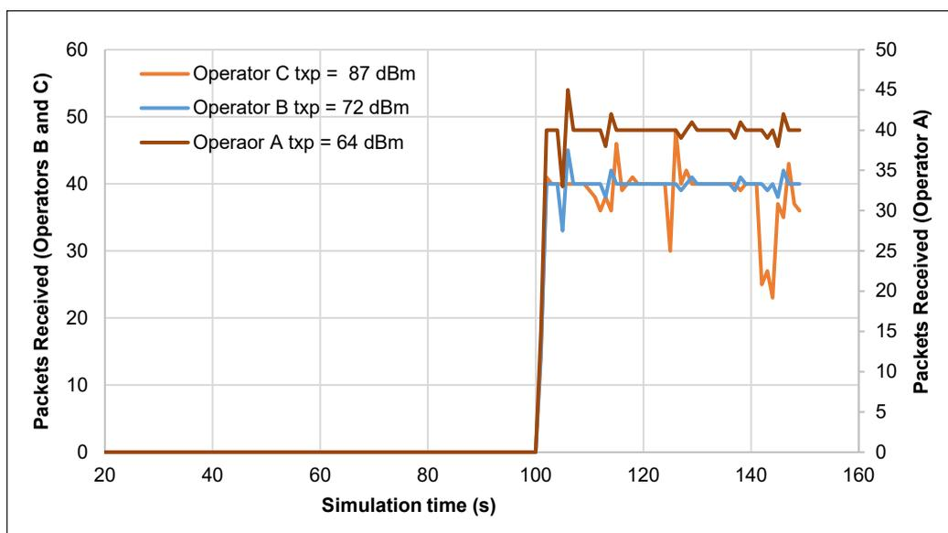
Figure 8. Comparison of the packets received based on the selected service provider for a typical node (50 nodes)
